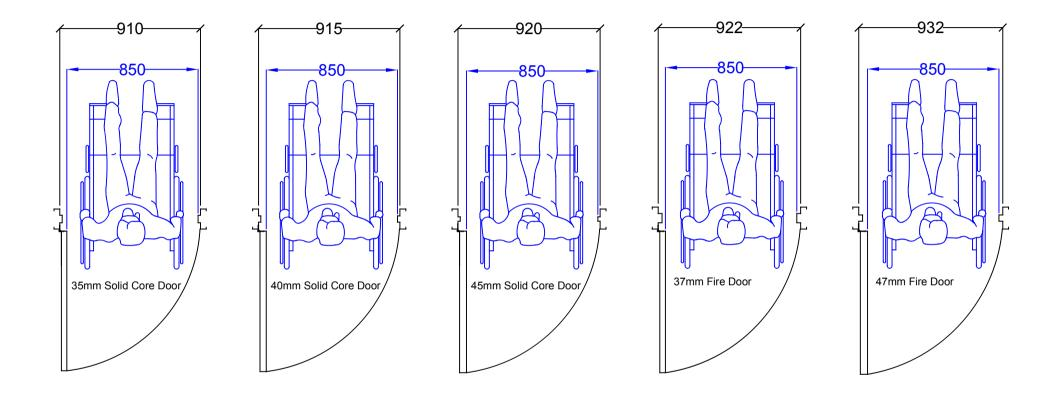
Minimum Clear Opening Reveal Size Recommendation - As Per Door Type and Thickness
